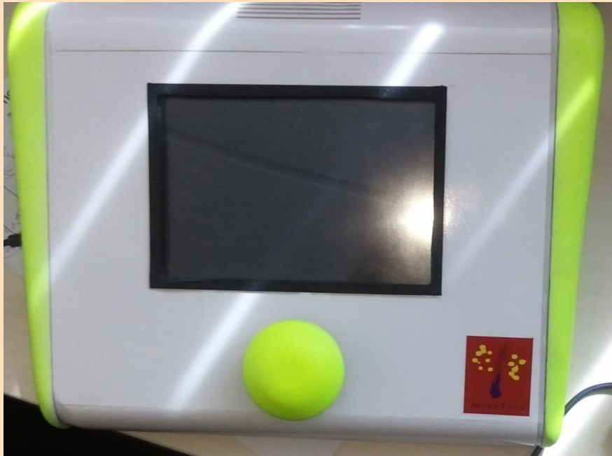
KAVI Version 1.0 Functional Prototype with 7.5" LCD Screen
